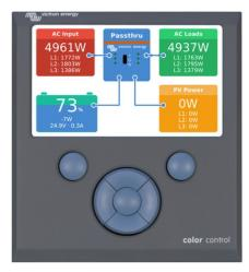
Color Control Panel, showing a PV application
